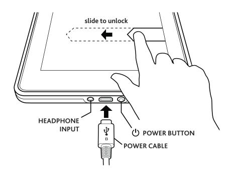
To charge your Kindle, connect it to the power cable as shown. Then connect the power adapter at the opposite end of the power cable into a wall outlet.
