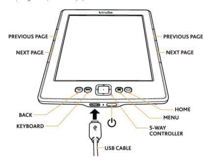
To the sides of the screen are the Next Page > and Previous Page < buttons. Both buttons are available on each side so you can hold your Kindle with either hand while reading.
