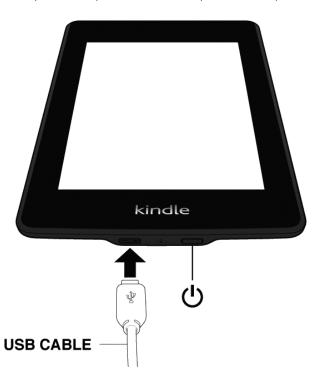
**Power button:** To turn your Kindle on, press the Power button. If you need to turn off your Kindle screen, press and hold the Power button for 7 seconds until the Power dialog displays and then select Screen Off.
